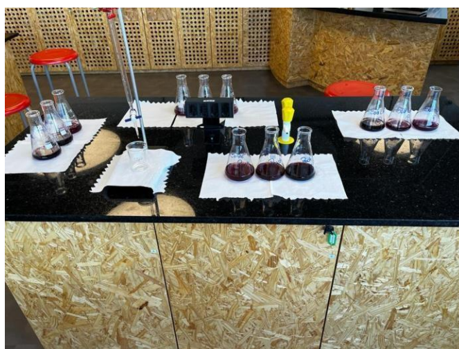
Figure 13: All the three samples of each Cachaça after reacting with Eriochrome black T. Elaborated by author.
