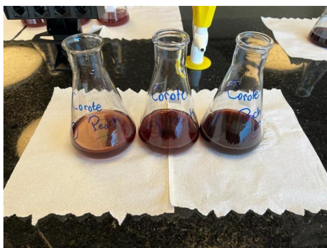
Figure 15: Three samples of Corote Peach after reacting with Eriochrome black T. Elaborated by author.
