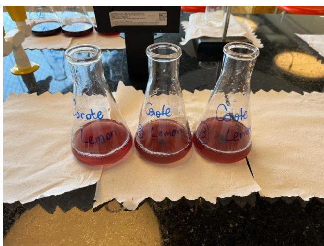
Figure 16: Three samples of Corote Lemon after reacting with Eriochrome black T. Elaborated by author.
