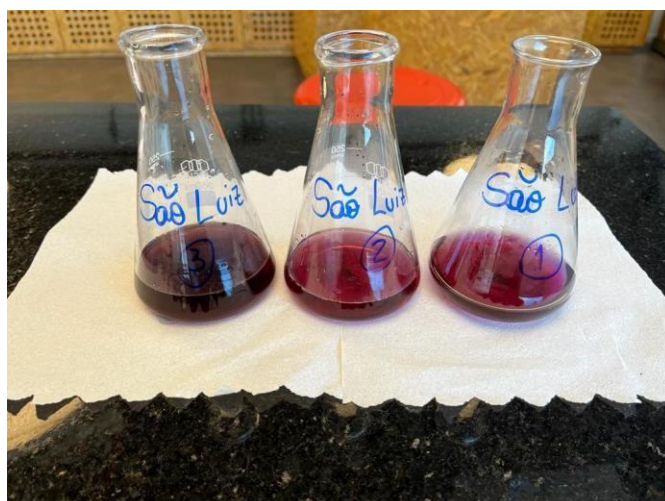
Figure 14: Three samples of Cachaça Engenho São Luiz after reacting with Eriochrome black T. Elaborated by author.
